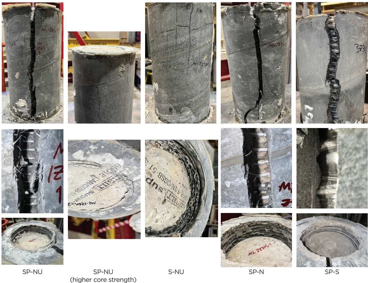
Figure 12. Failure modes of Z specimens.
