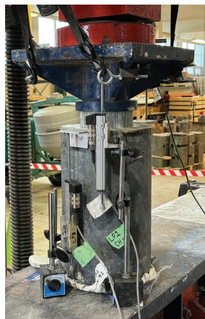
Figure 4. Push-out test setup. Note: LP = linear potentiometer; NSC = normal-strength concrete; SIFP = stay-in-place form; UHPC = ultra-high-performance concrete.
