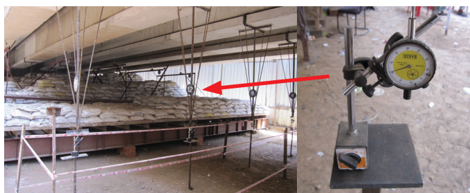
Arrangement for measuring girder deflection using dial gauges
