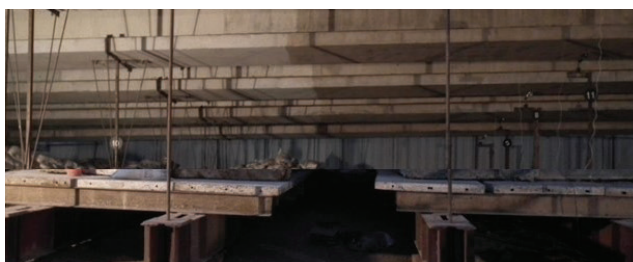
Platform with dead weights below the deck and arrangement for measuring girder deflection using dial gauges
