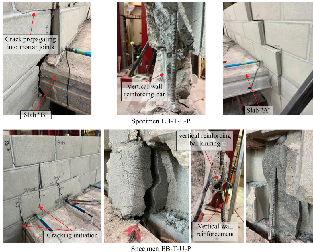
Figure 6. Test specimens at failure. Note: EB-T-L-P = end bearing configuration with tensile loading and an L-shaped bar connection with a parapet configuration; EB-T-U-P = end bearing configuration with tensile loading and a U-shaped bar connection with a parapet configuration.
