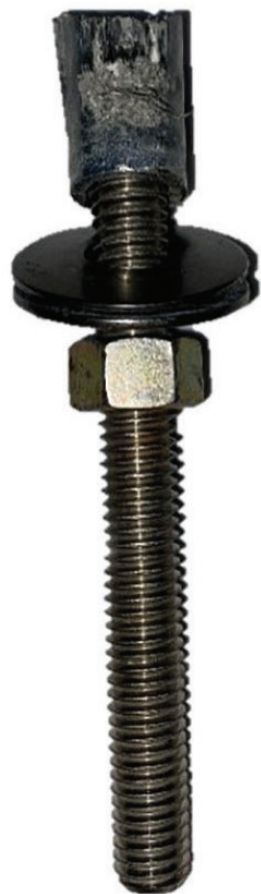
Failed connector with the attached threaded rod
