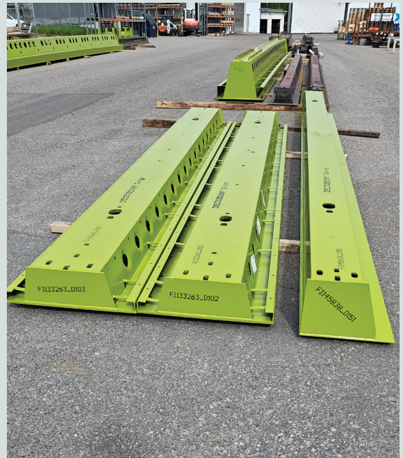
Complete Deltabeams await shipment at Peikko. Courtesy of Jason Lien.
