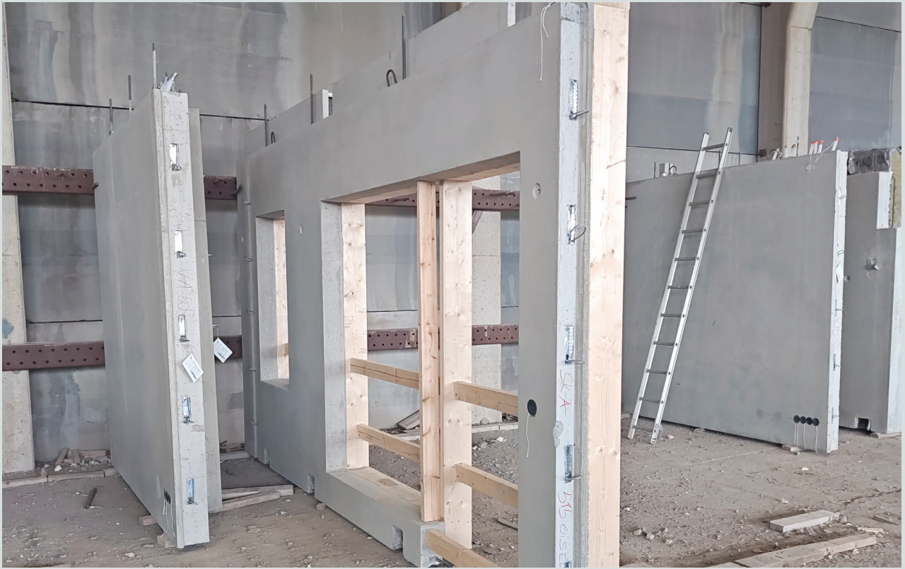
These panels in storage at Santalan Betoni are waiting for delivery. The final details, which have been completed, consisted of threading pull string through the electrical conduit. A unique blocking technique for the door jamb is used with cast-in reinforcing bar combined with a lumber tension strut to prevent movement of the jamb in storage and transport. This was a common stiffening technique throughout the plants visited. Courtesy of Jason Lien.
