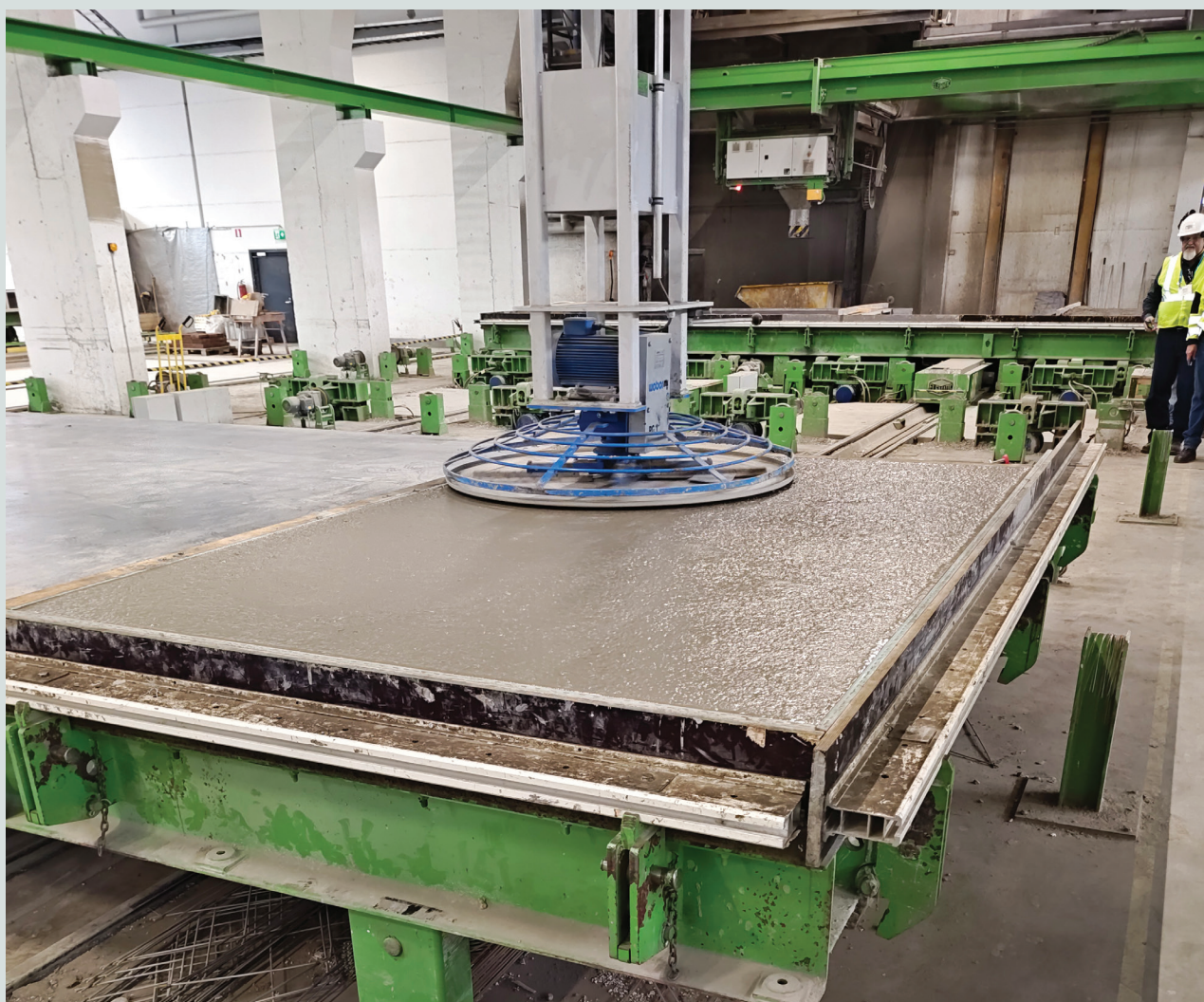
This carousel table at Santalan Betoni has a precast concrete panel on it. The top form surface is being finished using a finish machine that controls rotation velocity and pressure, and the operator is off to the side to guide the equipment and ensure safe operation. For the final detail, a finisher will only touch the edges of the panel. Courtesy of Jason Lien.
