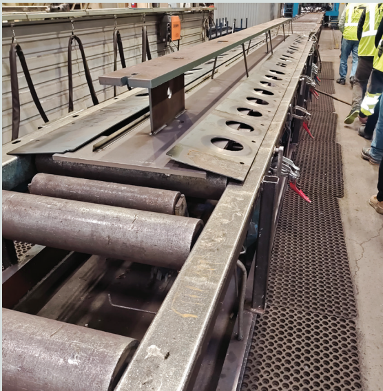
The top and bottom flanges of a Deltabeam at Peikko in Lahti, Finland, are separated by spacers while it waits for the installation of its side plates. The assembly is tacked together before inserting the beam into an automated welding machine to automatically weld each web and each flange simultaneously. Courtesy of Jason Lien.
