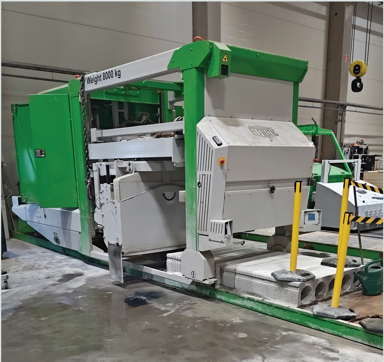
The final assembly of the hollow-core saw at Elematic in Akaa, Finland, is being used to make crosscuts to a test piece of hollow-core. Courtesy of Jason Lien.
