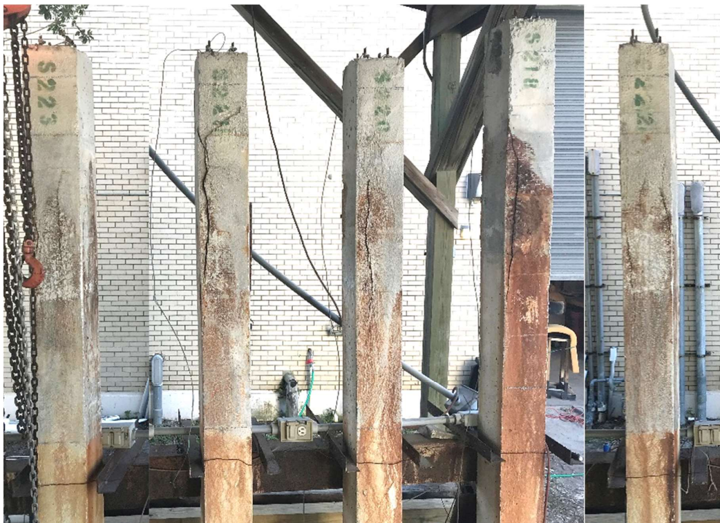
Figure 4. Condition of piles 1, 2, 3, 4, and 5 at the start of part 3 of the research program, 20 years after they were cast. The piles are shown from left to right, looking at the east side.
