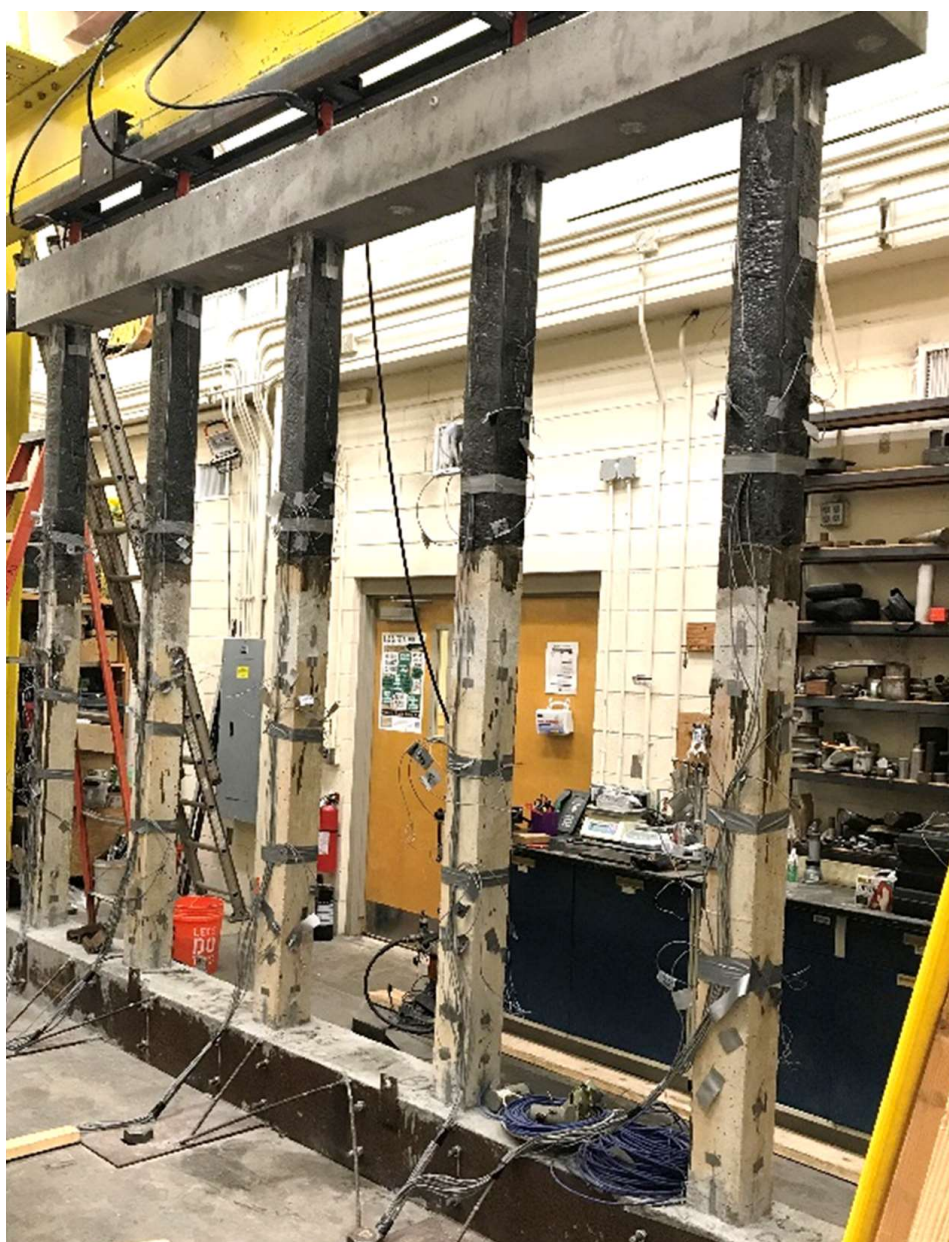
Figure 21. Fully instrumented pile bent.
