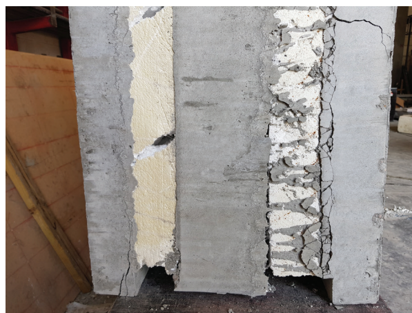
Exterior wythe bearing directly on the testing machine platen without bottom PTFE strips
