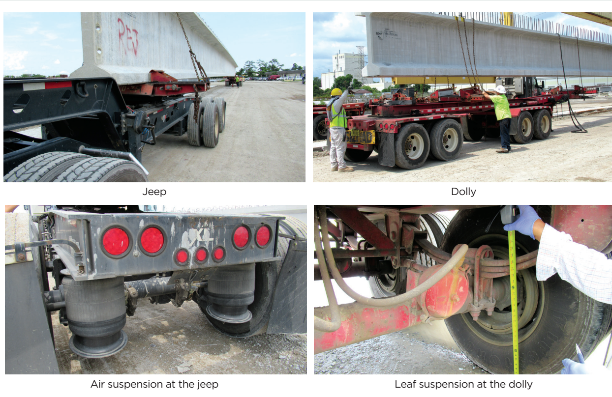
Figure 2. Views of the jeep and dolly setup.
