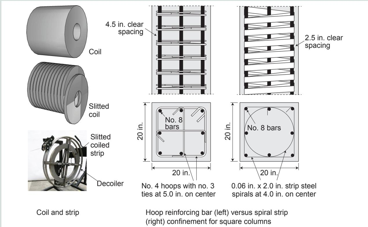
**Figure 1.** High-strength steel strip reinforcement. Note: no. 3 = 10M; no. 4 = 13M; no. 8 = 25M; 1 in. = 25.4 mm.
