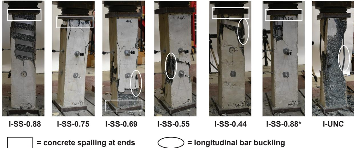
**Figure 10.** Phase I damage states after peak load but prior to residual load testing. Note: For specimen labels, the first term denotes test phase (I or II), the second term denotes confinement reinforcement type and layout (RH = reinforcing bar hoops, SS = strip spiral, SH = strip hoops, 2SS = two strip spirals, and UNC = unconfined), the third term denotes confinement volumetric ratio as a percentage, and an asterisk indicates alternative anchorage.
