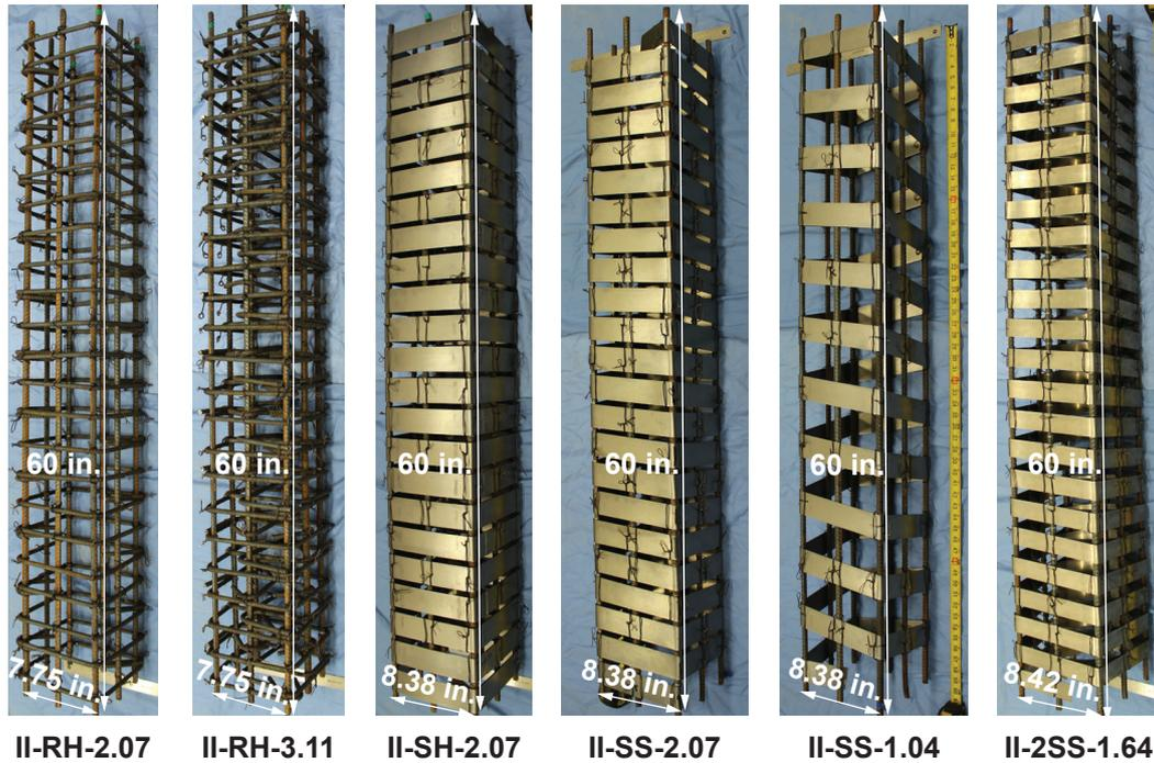
**Figure 7.** Phase II (10.0 × 10.0 in. [254 × 254 mm] cross section) column reinforcement cages prior to casting. Note: For specimen labels, the first term denotes test phase (I or II), the second term denotes confinement reinforcement type and layout (RH = reinforcing bar hoops, SS = strip spiral, SH = strip hoops, 2SS = two strip spirals, and UNC = unconfined), and the third term denotes confinement volumetric ratio as a percentage. 1 in. = 25.4 mm.
