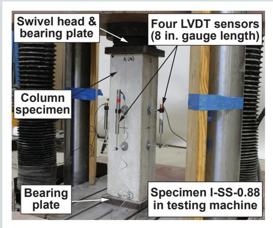
**Figure 5.** Phase I test setup and instrumentation. Note: For specimen labels, the first term denotes test phase (I or II), the second term denotes confinement reinforcement type and layout (RH = reinforcing bar hoops, SS = strip spiral, SH = strip hoops, 2SS = two strip spirals, and UNC = unconfined), and the third term denotes confinement volumetric ratio as a percentage. LVDT = linear variable displacement transducer.
