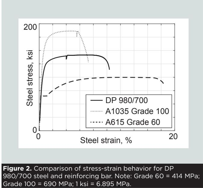
**Figure 2.** Comparison of stress-strain behavior for DP 980/700 steel and reinforcing bar. Note: Grade 60 = 414 MPa; Grade 100 = 690 MPa; 1 ksi = 6.895 MPa.
