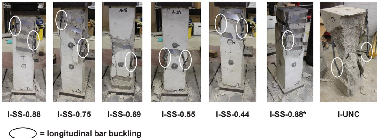
**Figure 11.** Phase I final column damage states after residual load testing. Note: For specimen labels, the first term denotes test phase (I or II), the second term denotes confinement reinforcement type and layout (RH = reinforcing bar hoops, SS = strip spiral, SH = strip hoops, 2SS = two strip spirals, and UNC = unconfined), the third term denotes confinement volumetric ratio as a percentage, and an asterisk indicates alternative anchorage.
