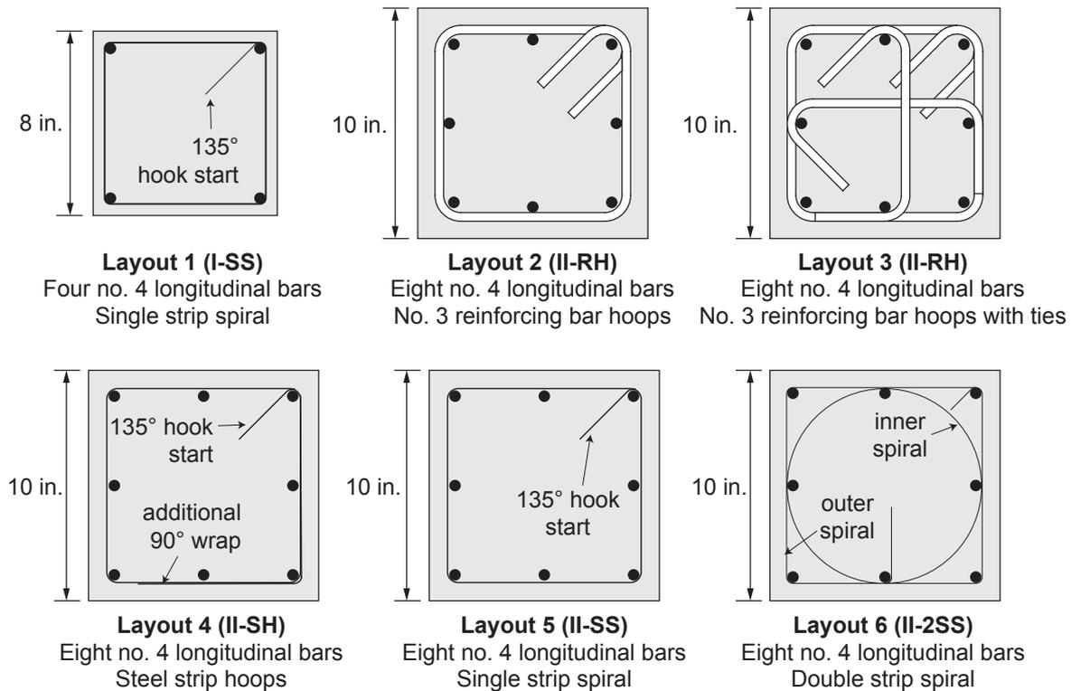
**Figure 4.** Column confinement layouts. Note: For specimen labels, the first term denotes test phase (I or II), and the second term denotes confinement reinforcement type and layout (RH = reinforcing bar hoops, SS = strip spiral, SH = strip hoops, 2SS = two strip spirals, and UNC = unconfined). No. 3 = 10M; no. 4 = 13M; 1 in. = 25.4 mm.
