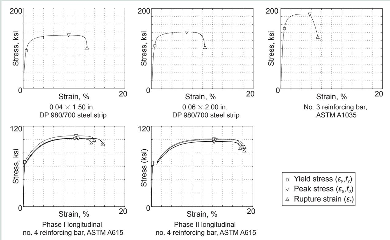
**Figure 8.** Measured reinforcing steel stress versus strain behavior. Note:  $f_u$  = peak steel strength;  $f_y$  = yield strength;  $\epsilon_r$  = steel rupture strain;  $\epsilon_u$  = steel strain at peak strength;  $\epsilon_y$  = steel strain at yield. No. 3 = 10M; no. 4 = 13M; 1 in. = 25.4 mm; 1 ksi = 6.895 MPa.
