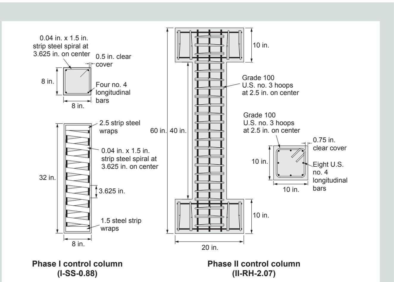
**Figure 3.** Phase I and II control columns (I-SS-0.88 and II-RH-2.07). Note: For specimen labels, the first term denotes test phase (I or II), the second term denotes confinement reinforcement type and layout (RH = reinforcing bar hoops, SS = strip spiral, SH = strip hoops, 2SS = two strip spirals, and UNC = unconfined), and the third term denotes confinement volumetric ratio as a percentage. Grade 100 = 690 MPa; no. 3 = 10M; and no. 4 = 13M; 1 in. = 25.4 mm.
