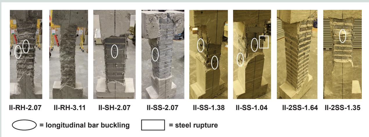
**Figure 12.** Phase II final column damage states. Note: For specimen labels, the first term denotes test phase (I or II), the second term denotes confinement reinforcement type and layout (RH = reinforcing bar hoops, SS = strip spiral, SH = strip hoops, 2SS = two strip spirals, and UNC = unconfined), and the third term denotes confinement volumetric ratio as a percentage.
