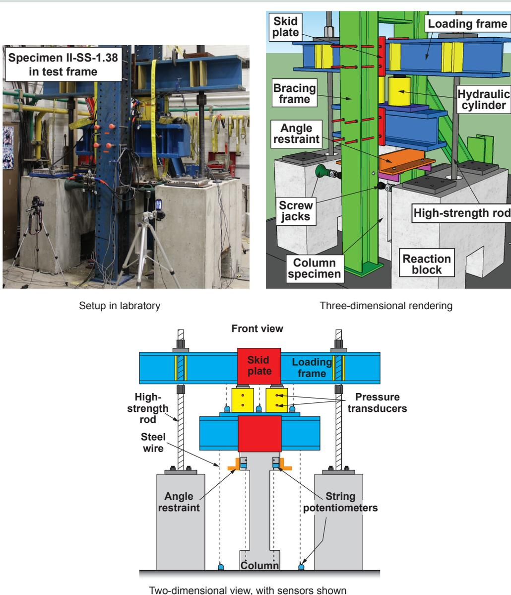
**Figure 6.** Phase II test setup and instrumentation. Note: For specimen labels, the first term denotes test phase (I or II), the second term denotes confinement reinforcement type and layout (RH = reinforcing bar hoops, SS = strip spiral, SH = strip hoops, 2SS = two strip spirals, and UNC = unconfined), and the third term denotes confinement volumetric ratio as a percentage.
