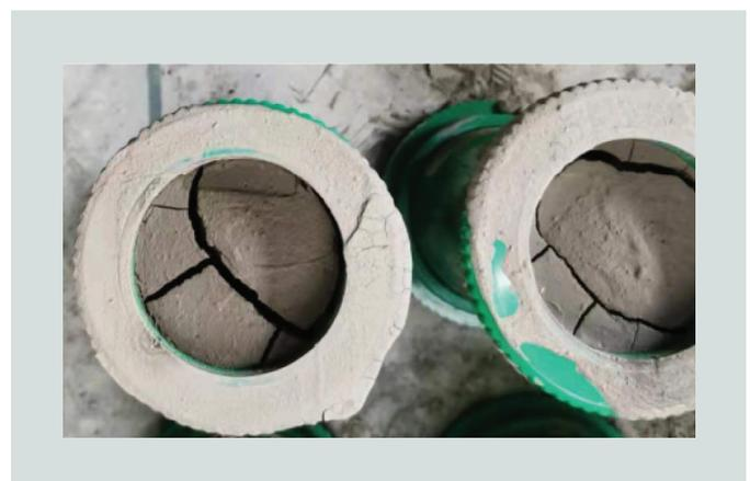
**Figure 2.** Shrinkage and cracking of dried lake sediments.
