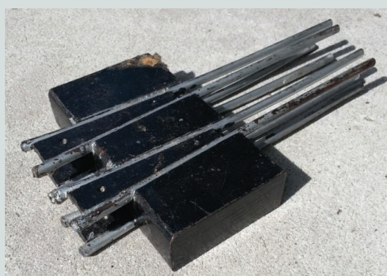
Eight-wire sandwich plate anchorage retrieved after demolition. Courtesy of Helmuth Wilden.
