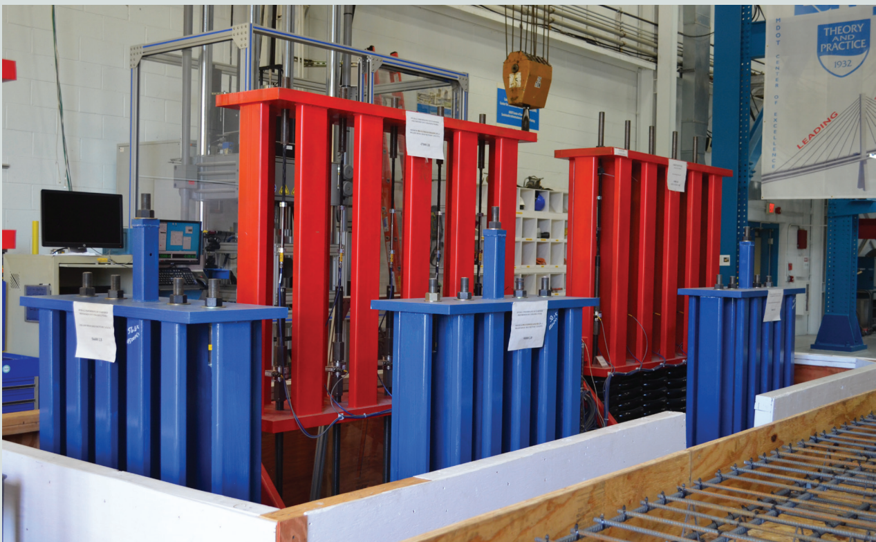
Figure 8. Stressed carbon-fiber-composite-cable specimens stored in a controlled laboratory environment.
