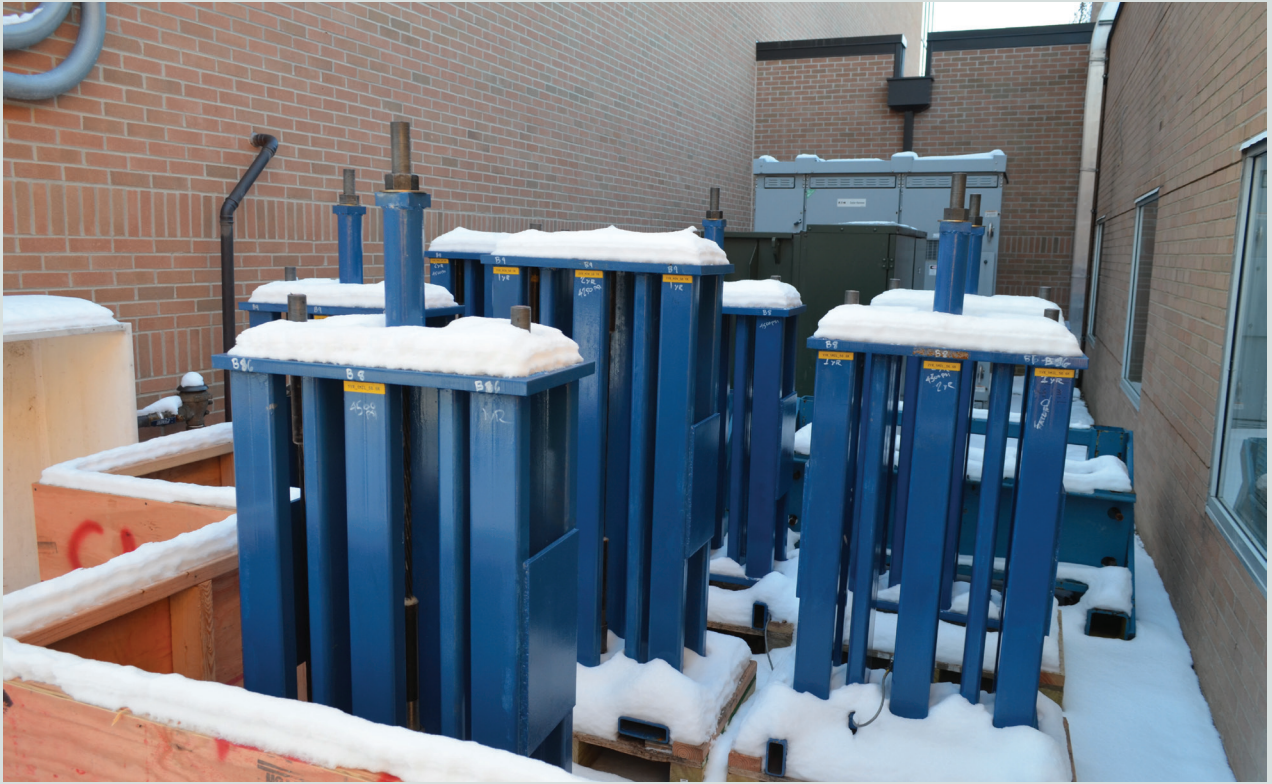
Figure 9. Stressed carbon-fiber-composite-cable specimens exposed to weather conditions.
