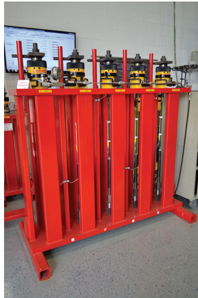
0.6 in. diameter CFCC with a closed-loop hydraulic system
