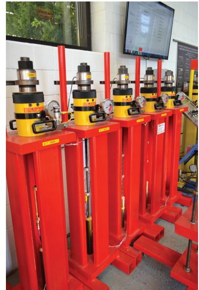
0.7 in. diameter CFCC with a closed-loop hydraulic system
