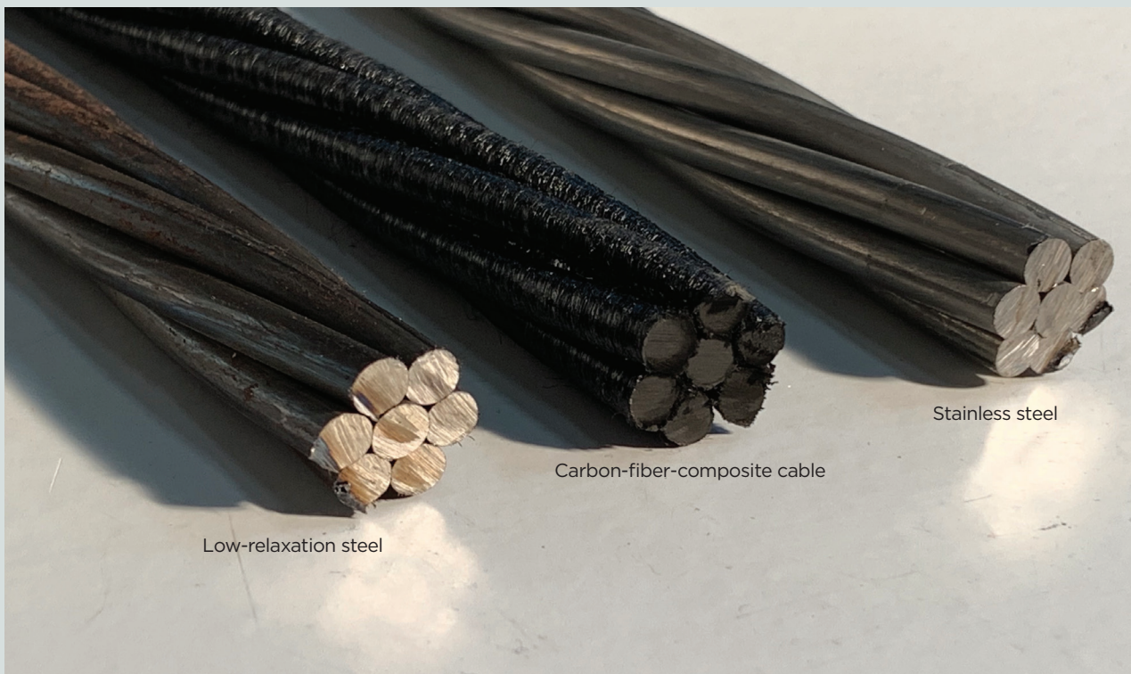
Figure 1. Cross-sectional views of 0.6 in. (15 mm) diameter low-relaxation steel, carbon-fiber-composite cable, and stainless steel prestressing strands.
