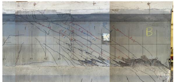
Failure mode: sliding shear at web-flange interface
