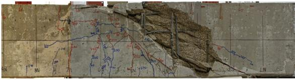
Failure mode: shear compression
