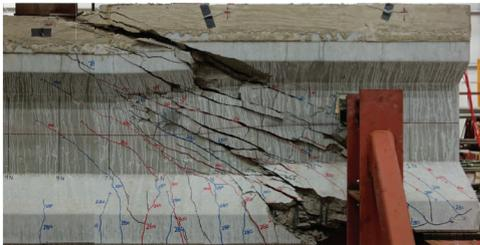
Failure mode: shear compression
