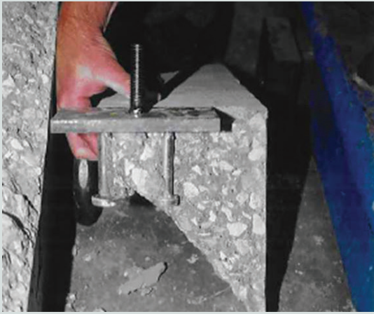
Shear failure of the stud group is controlled by the distance of the rear stud(s) from the free edge. Source: Reproduced from Anderson, Tureyen, and Meinheit (2007), Fig. 7.4.1.
