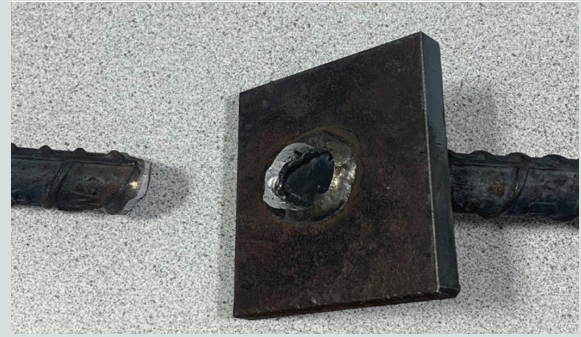
Figure 6. Test sample showing fracture surface. Reproduced by permission from Michael Kerr.
