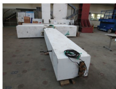
Prestressing of steel tendons
