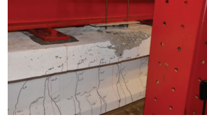
Figure 12. Crack distribution and failure mode of test beams at ultimate load. Note: P = applied load. 1 in. = 25.4 mm.
