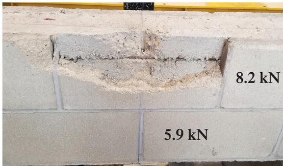
Masonry beam cracking and cover spalling (EB-TN-D)
