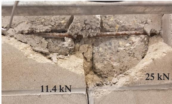
Masonry beam cracking and spalling (EB-CN-A)
