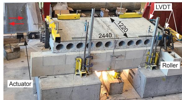
Parallel load on end-bearing specimen
