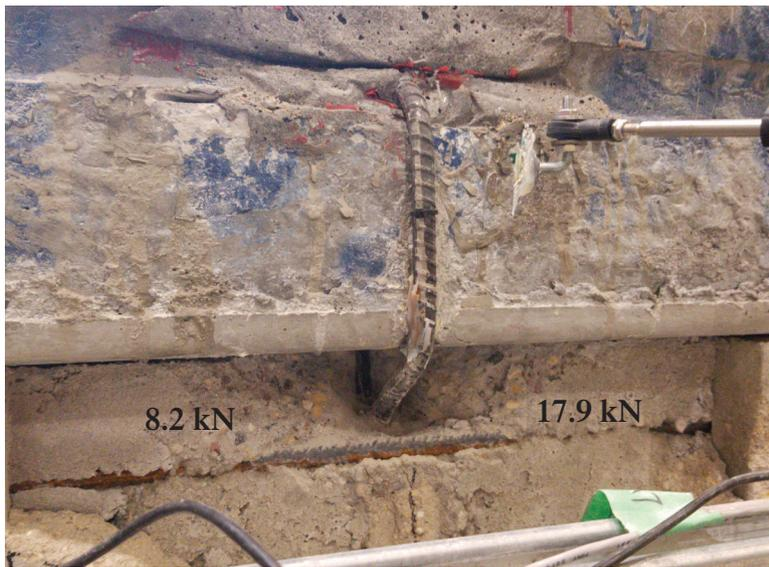
Masonry beam cracking (SB-CN-D)
