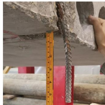
Bar deformation and pull-out (EB-TN-D)
