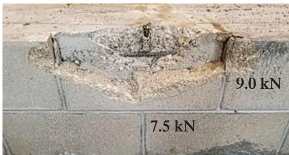
Masonry beam cracking and spalling (EB-TN-A)
