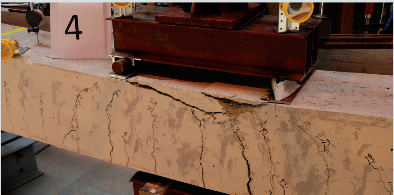
Figure 5. Simply supported beam with bonded tendons (beam 4) at failure.
