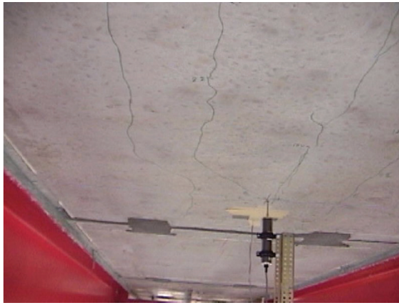
Figure 13. Observed cracks in experimental testing. Source: Reproduced by permission from Issa et al. (2007, Fig. 12 and 16).
