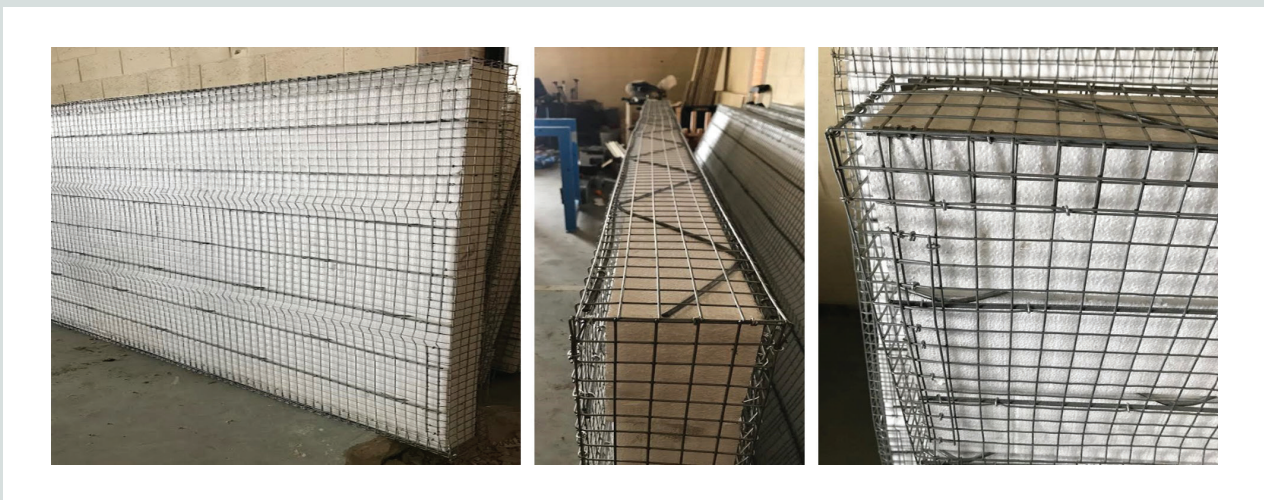
Figure 7. Modular structural concrete insulated panel cores without additional reinforcement in the splice zones.
