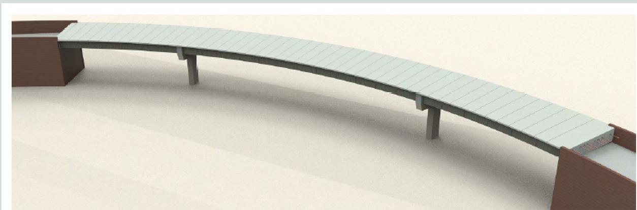
**Figure 13.** Three-dimensional model of the three-span (120, 240, and 120 ft), 50 ft wide bridge with a horizontal curvature radius of 500 ft. The total superstructure, including the 10 ft wide deck, is made of precast concrete components. Note: 1 ft = 0.305 m.
