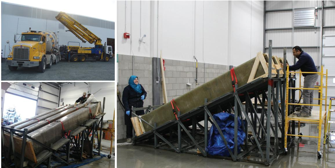
Beam casting setup and casting
