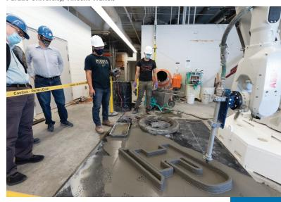
materials that we want to use for large-scale construction in marine environments," Rodriguez says. "The current robotic system will allow us to produce larger elements on which we can evaluate properties such as their strength and durability."
