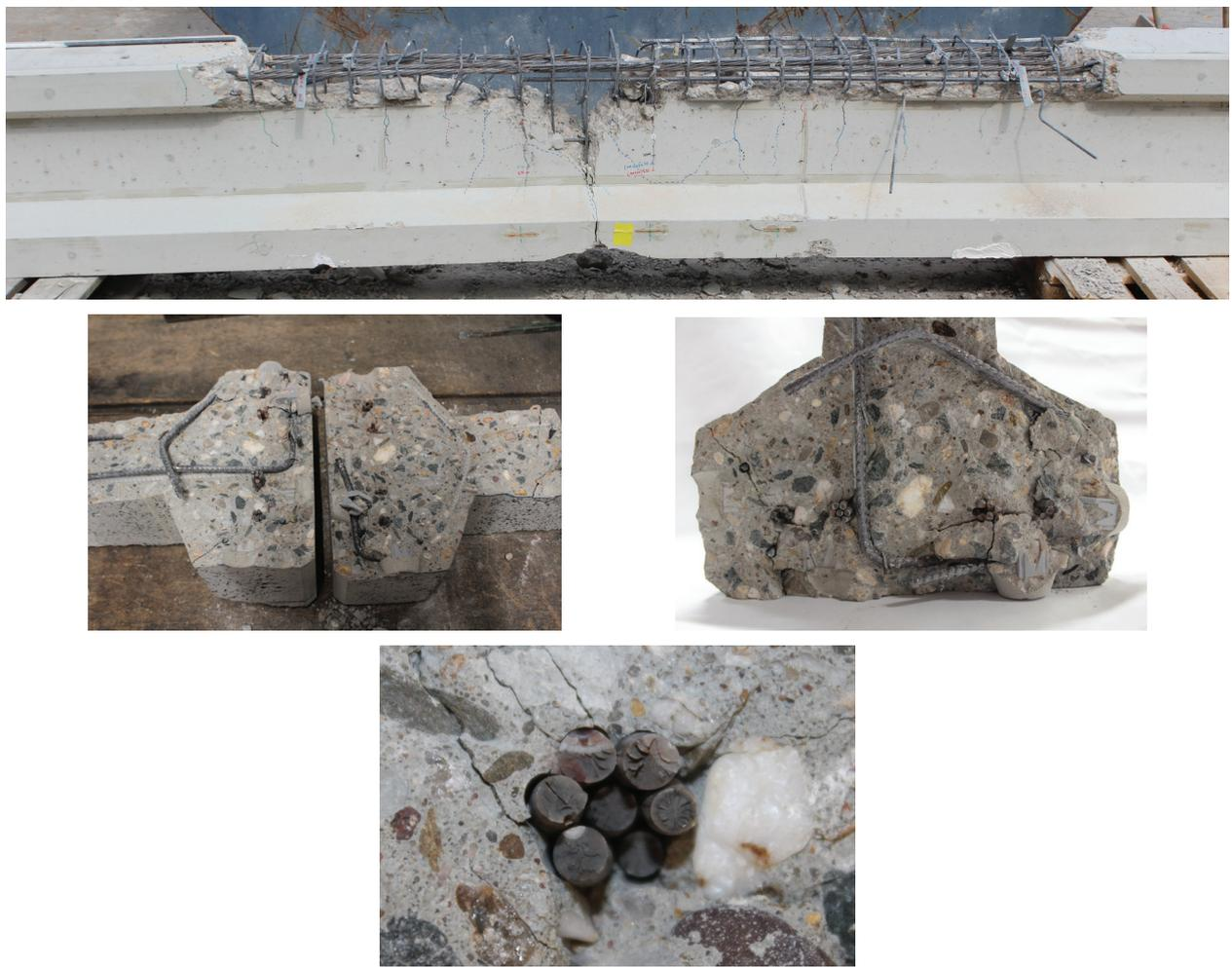
**Figure 11.** Dismantling of strands in bottom flange of beam B7 after failure.
