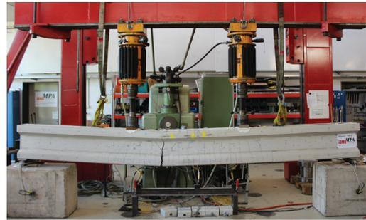
Beam B7 after fatigue failure
