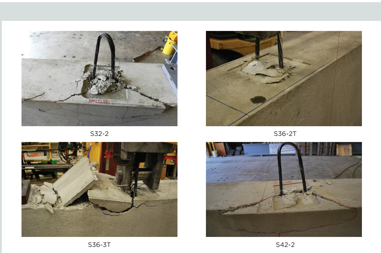
Figure 10. Failure modes of straight loop test specimens. Note: S32-2 = second test in straight loop test series with 32 in. embedment depth; S36-2T = second test in straight loop test series with 36 in. embedment depth; S36-3T = third test in straight loop test series with 36 in. embedment depth; S42-2 = second test in straight loop test series with 42 in. embedment depth. 1 in. = 25.4 mm.
