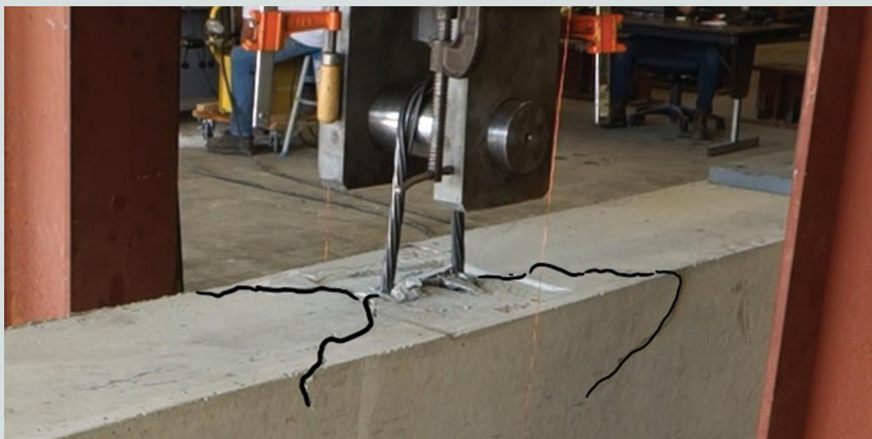
Figure 8. Initial cracking for B24-2. Cracks have been emphasized (traced) for clarity. Note: B24-2 = second test in bent loop test series with 24 in. embedment depth. 1 in. = 25.4 mm.
