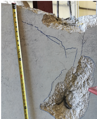
Close-up of side face blowout in B30-1
