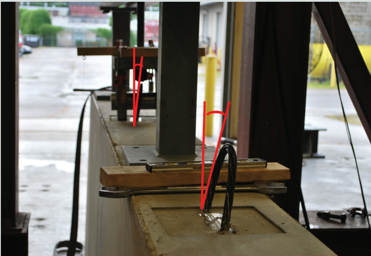
Figure 6. Inclined position of B30 loops. Note: B30 = bent loop test series with 30 in. embedment depth. 1 in. = 25.4 mm.
