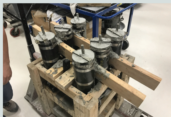
Figure 7. Stainless steel specimens prepared for bond test.
