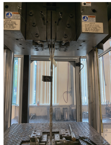
Strand at failure
