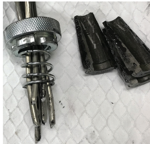
Notching effect of grips on the stainless steel strands
