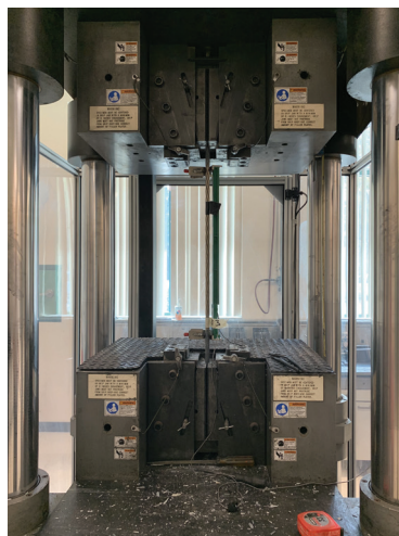
Extensometer attached to a strand to measure strain up to 1% elongation
