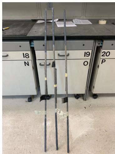
Specimens prepared for tensile testing
