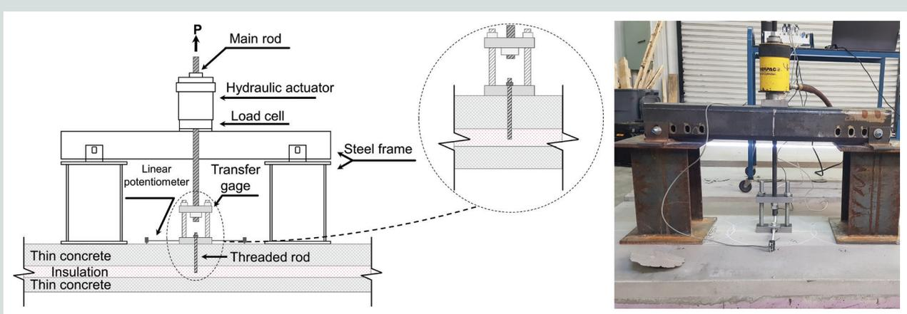
**Figure 6.** Test apparatus. Note: P = applied load. 1 in. = 25.4 mm.
