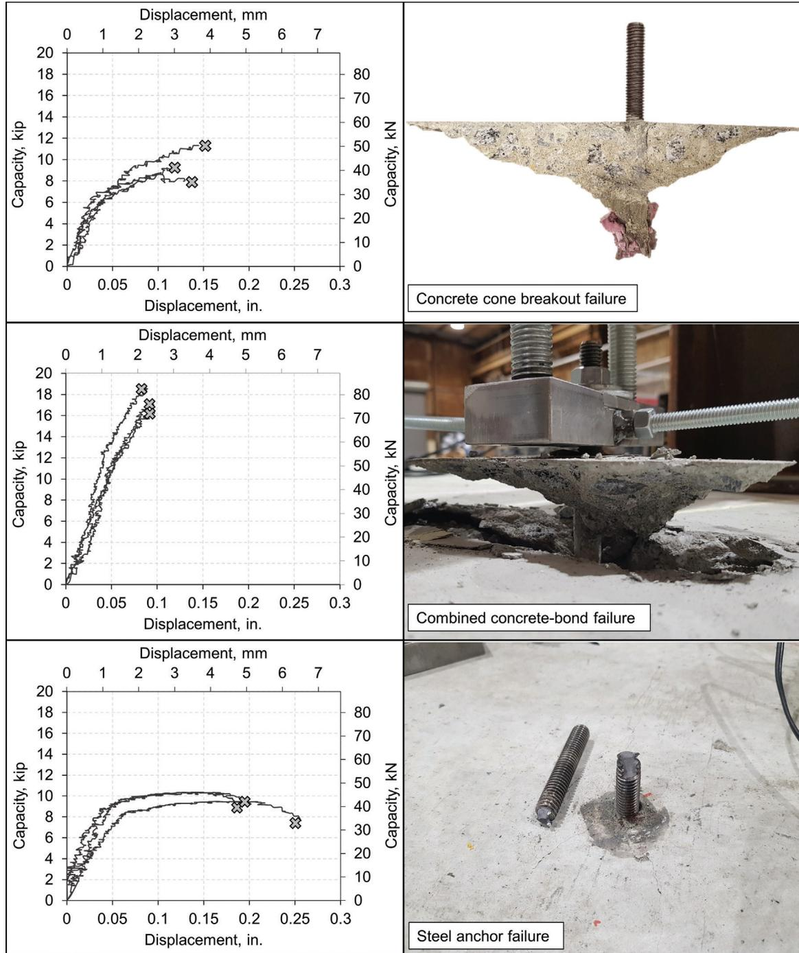
**Figure 7.** Load-displacement and failure mode for concrete cone breakout failure, combined concrete-bond failure, and steel anchor failure.
