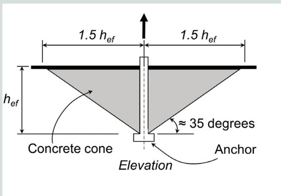
**Figure 3.** Concrete capacity design model. Note:  $h_{ef}$  = effective anchor embedment depth.
