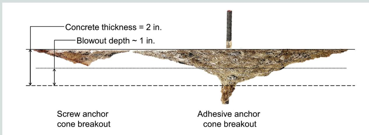
**Figure 10.** Adhesive and screw anchors concrete cone breakout. Note: 1 in. = 25.4 mm.
