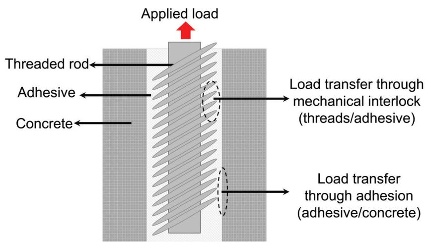
**Figure 1.** Adhesive anchor load transfer mechanism.
