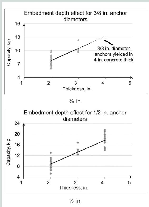
**Figure 9.** Concrete thickness effect on anchor capacity for 3/8 and 1/2 in. diameter anchor. Note: 1 in. = 25.4 mm; 1 kip = 4.448 kN.
