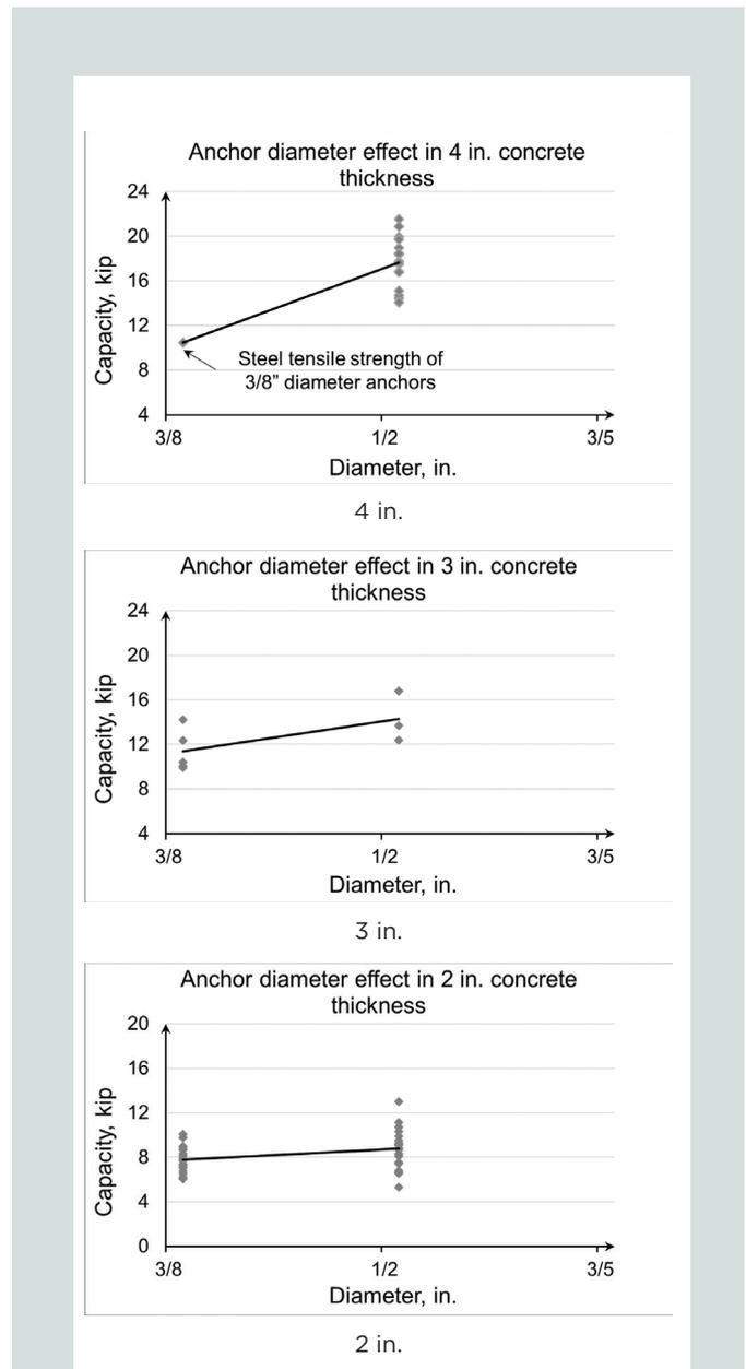
Figure 8. Anchor diameter effect in 4, 3, and 2 in. concrete thickness. Note: 1" = 1 in. = 25.4 mm; 1 kip = 4.448 kN.
