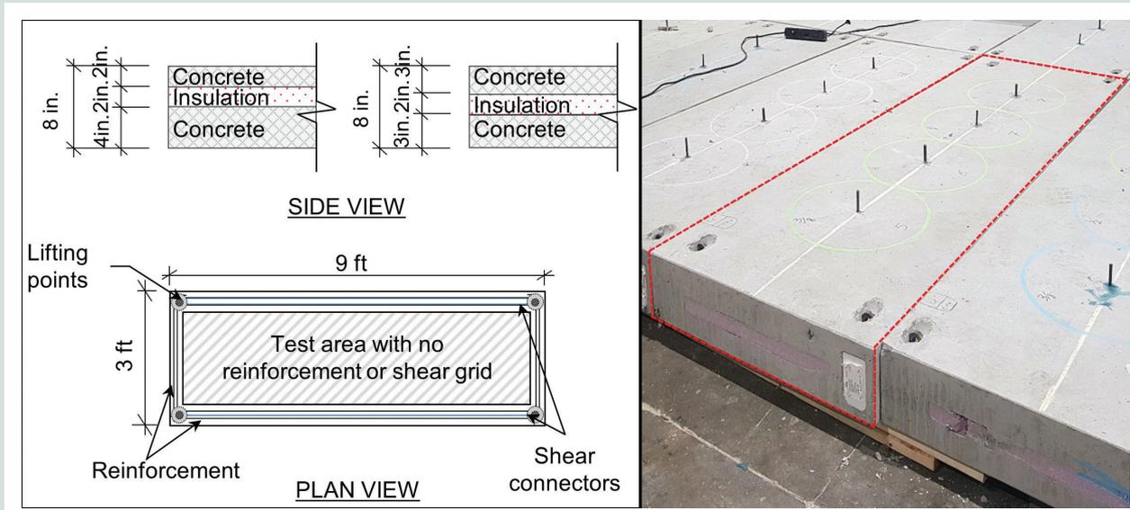
**Figure 5.** Side and plan view for the tested precast concrete sandwich panels. Note: 1 in. = 25.4 mm; 1 ft = 0.305 m.
