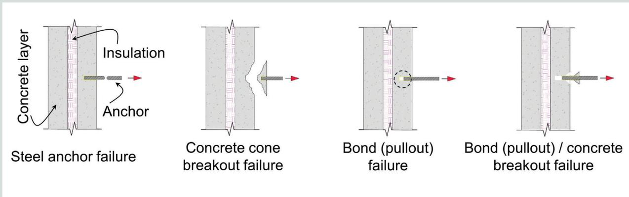
**Figure 2.** Failure modes for anchors embedded in one layer of precast concrete sandwich panel system.
