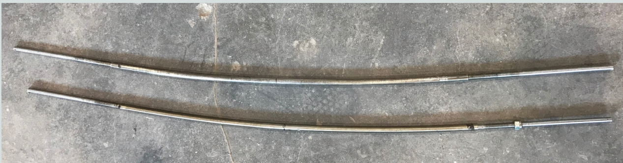
Figure 15. Shape memory alloy rod condition after reuse.
