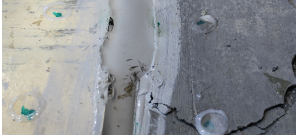
Concrete spalling from the top surface of the test panel
