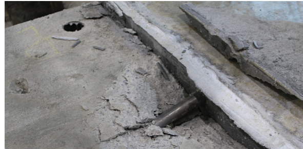
Concrete spalling from the top surface of the test panel
