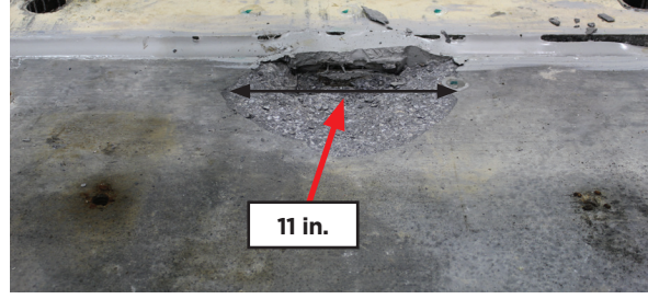
Concrete spalling from the top surface of the test panel
