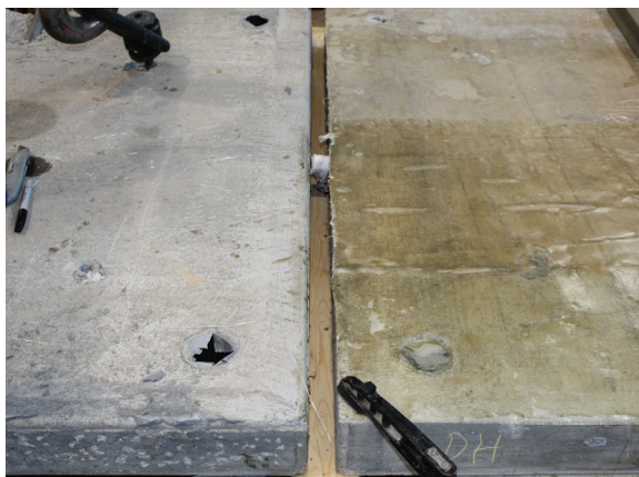
Inserting shape memory alloy rod in both panels
