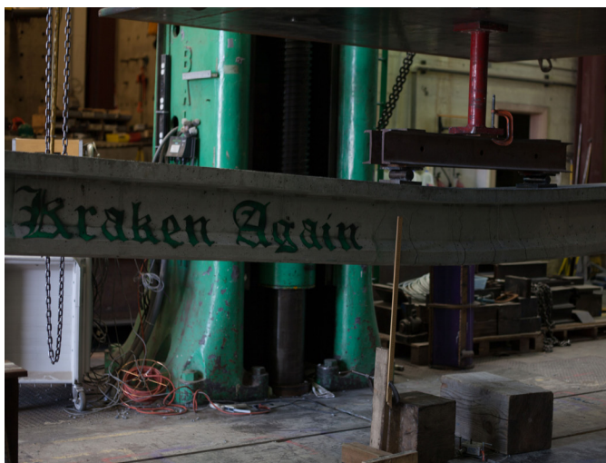
The 2017 Saint Martin's University PCI Big Beam Contest entry is shown between cracking and ultimate load during testing at the University of Washington. Courtesy of Clarinda Marion.
