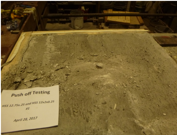
Figure 13. Failure mode of mechanically connected shear pocket connections.
