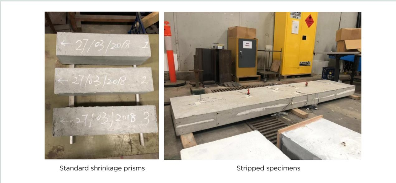
**Figure 3.** Shrinkage tests.
