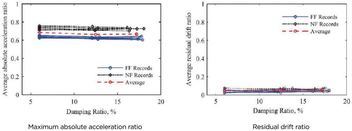
**Figure 12.** Average response ratios of the calculated maximum values to the allowable limits. Note: FF = far-field ground motion; NF = near-field ground motion.
