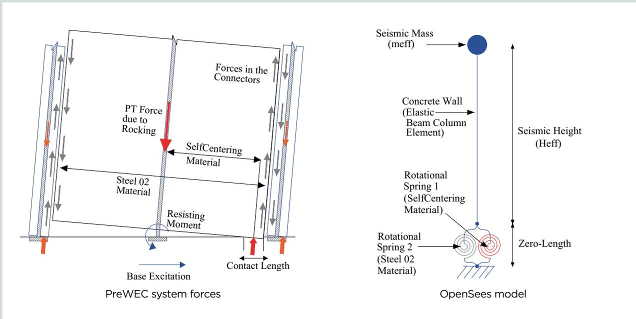
**Figure 7.** Forces contributing to base moment resistance in a PreWEC system and the corresponding OpenSees model. Source: Reproduced by permission from Nazari and Sritharan (2018). Note: PreWEC = precast concrete wall with end columns; PT = post-tensioning.
