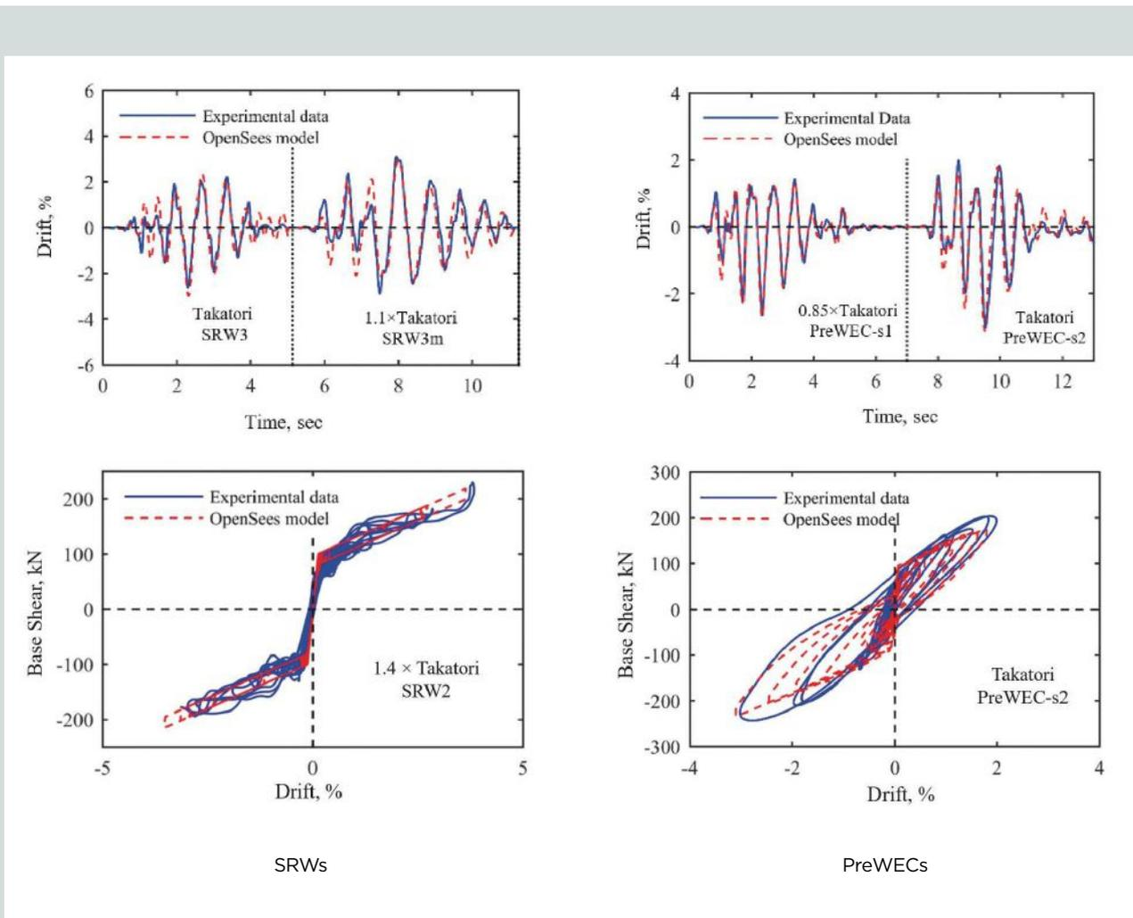
**Figure 8.** Experimental verification of the OpenSees models of SRWs and PreWECs. Source: Data for left graphs (top and bottom) from Nazari, Sritharan, and Aaleti (2016); data for right graphs (top and bottom) from Nazari and Sritharan (2018). Note: 1 kN = 0.225 kip. Note: PreWEC = precast concrete wall with end columns; SRW = single rocking wall.
