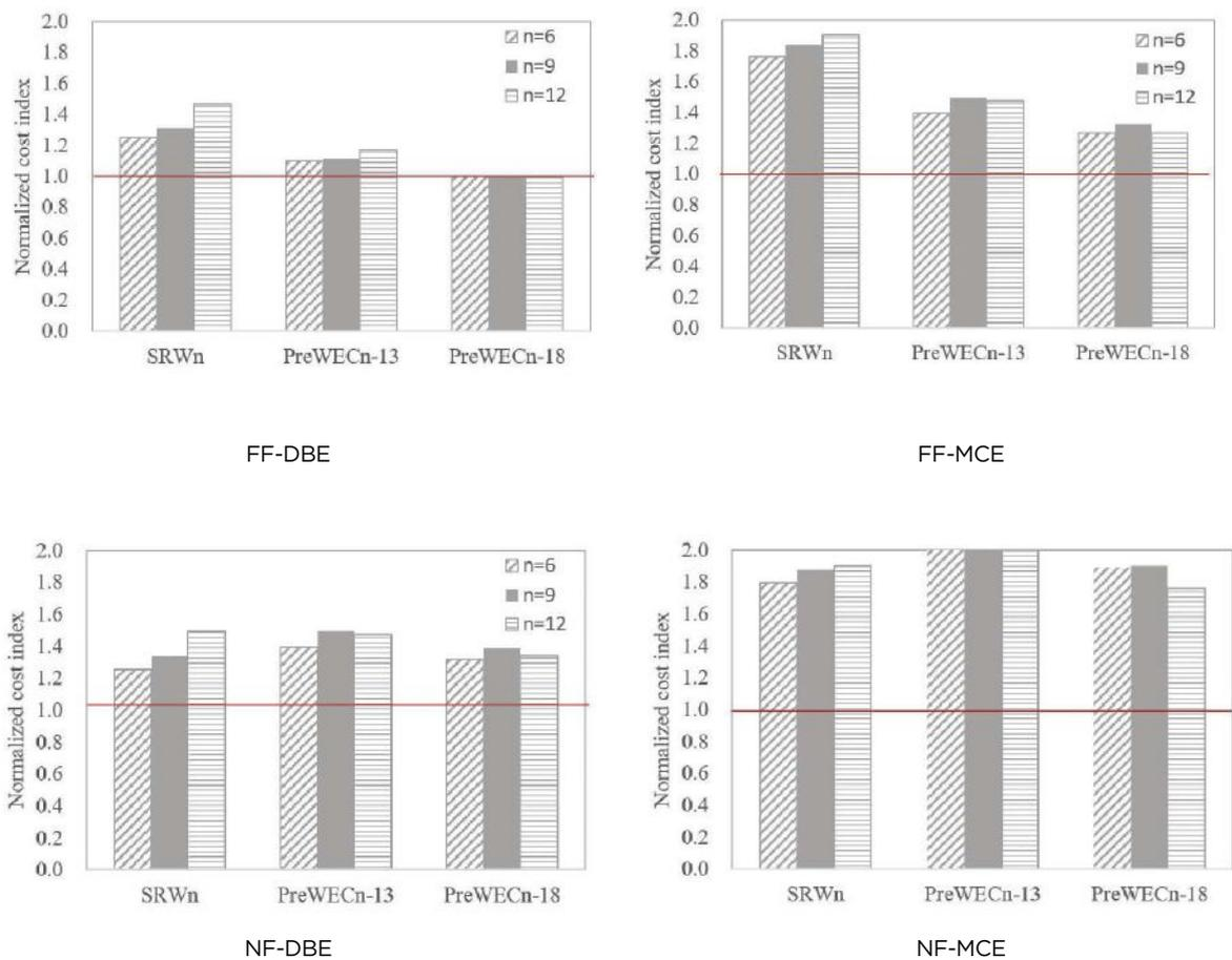
**Figure 13.** Normalized cost index for different case study buildings. Note: DBE = design-basis earthquake; FF = far-field ground motion; MCE = maximum considered earthquake;  $n$  = number of stories in the case study buildings; NF = near-field ground motion; PreWEC = precast concrete wall with end columns; SRW = single rocking wall.
