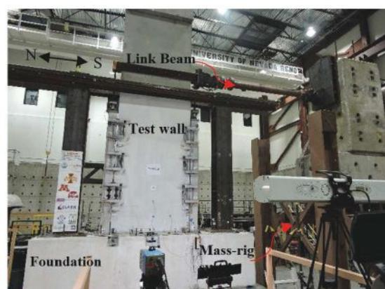
Precast concrete wall with end columns
