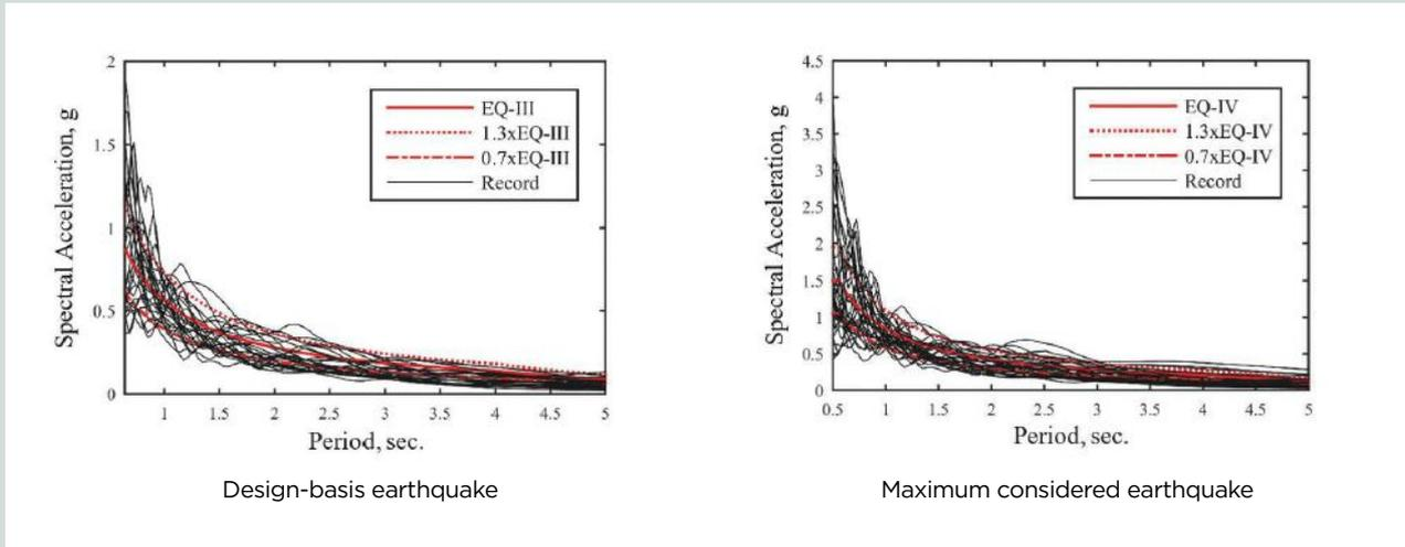
**Figure 6.** Spectral acceleration of scaled near-field and far-field ground motion records selected for analysis. Note: EQ-III = seismic hazard level III, representing design-basis earthquake events; EQ-IV = seismic hazard level IV, representing maximum considered earthquake events;  $g$  = acceleration of gravity.
