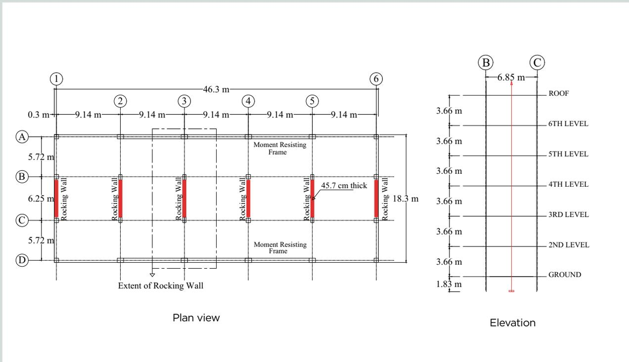
**Figure 5.** Plan view of buildings and elevation of a six-story building. Note: 1 cm = 0.394 in.; 1 m = 3.28 ft.
