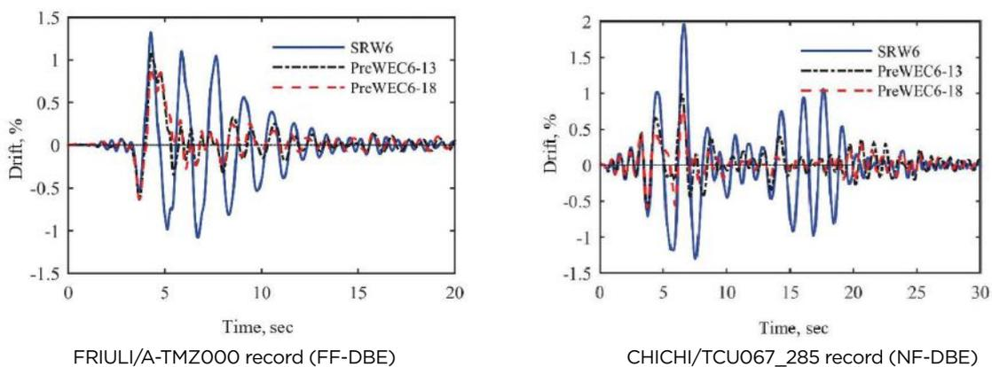
**Figure 9.** Impact of additional hysteretic damping on the drift time history response for two earthquake records. Note: DBE = design-basis earthquake; FF = far-field ground motion; NF = near-field ground motion; PreWEC = precast concrete wall with end columns; SRW = single rocking wall.
