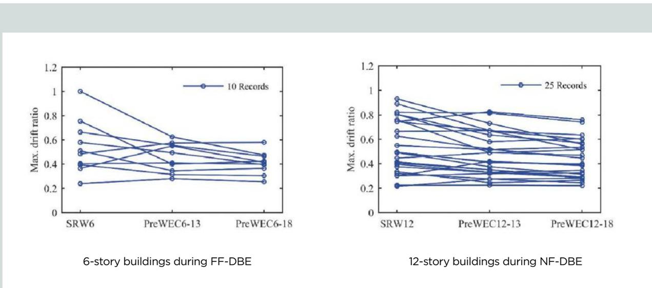
Figure 10. Ratio of the maximum drift to the allowable limit  $d_{max}$ . Note: DBE = design-basis earthquake; FF = far-field ground motion; NF = near-field ground motion; PreWEC = precast concrete wall with end columns; SRW = single rocking wall.
