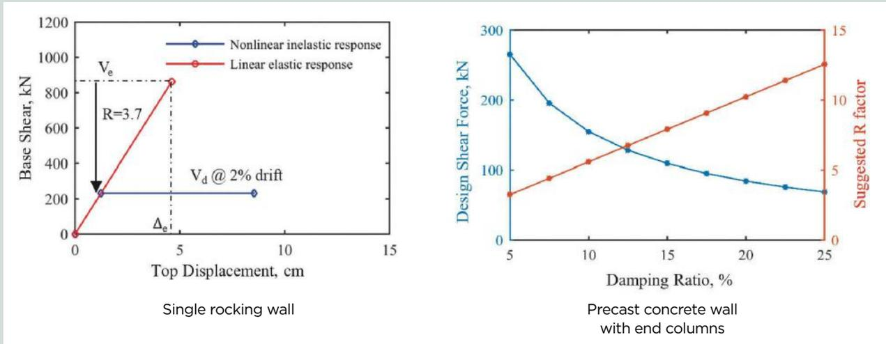
**Figure 4.** R factors suggested for force-based design of precast concrete rocking wall systems—FF records. Source: Data for right graph from Nazari and Sritharan (2018). Note: FF = far-field motion; R = response modification coefficient;  $V_d$  = design-level shear resistance;  $V_e$  = base shear force corresponding to the elastic response of the system;  $\Delta_e$  = elastic response displacement. 1 cm = 0.394 in.; 1 kN = 0.225 kip.
