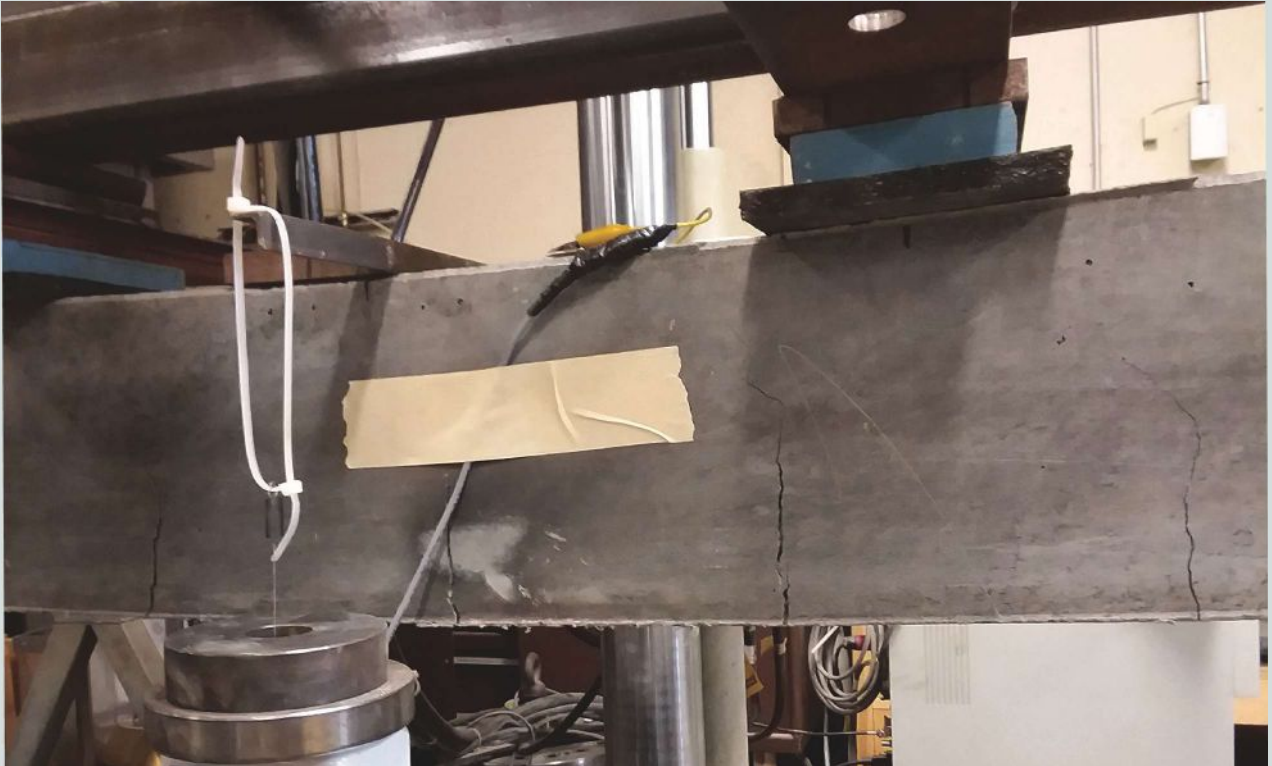
Figure 7. Crack pattern during beam configuration 2 experiment.
