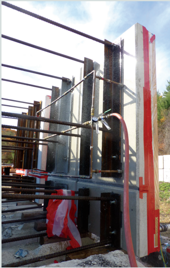
Figure 8. Test panel assembly water spray side.
