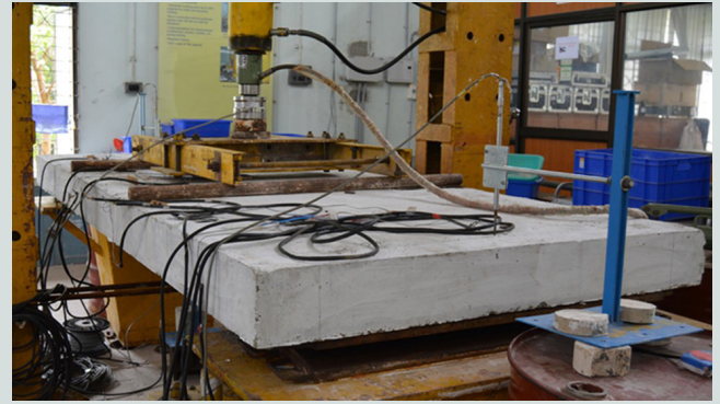
Figure A6. Four-point bending test setup.
