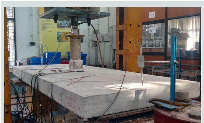
Figure A7. Punching test setup.
