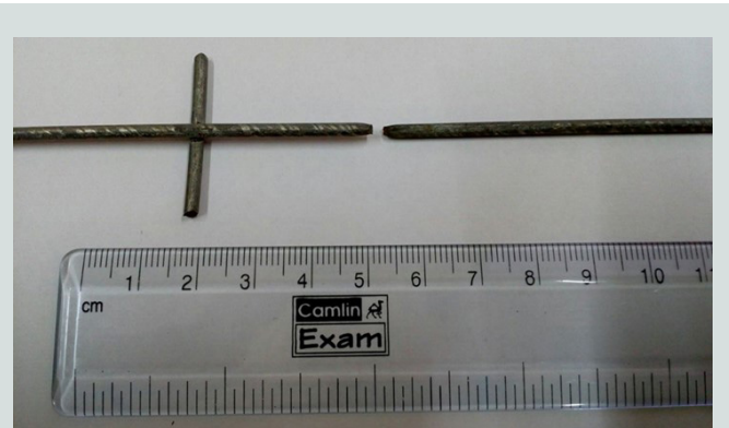
Figure A2. Tested mesh wire after failure.
