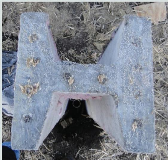
**Figure 6.1.** Ultra-high-performance concrete pile end after driving.
