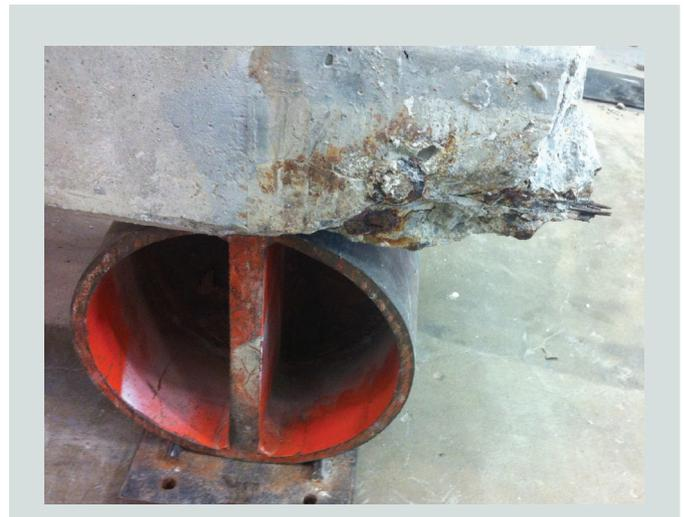
**Figure 3.** Corrosion at tested end for test A1.
