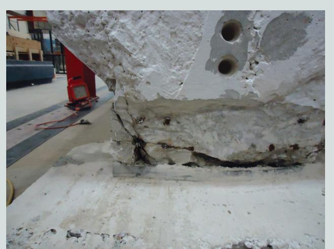
**Figure 7.** Spalling under load during test C1 initiated by cracking caused by corrosion.
