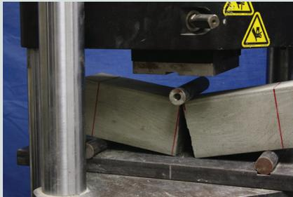
Modulus-of-rupture test setup
