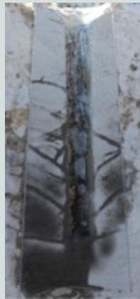
Cracks at middle and bottom of sleeve (Specimen 8)
