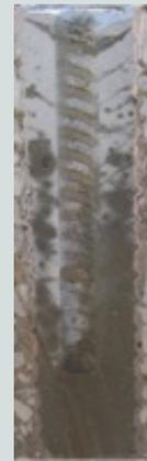
Cracks at top and middle of sleeve, with essentially no cracking at bottom (Specimen 9)
