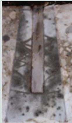
Cracks at middle and bottom of sleeve, with essentially no cracking at top (Specimen 7)
