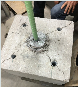
Figure 14. Mode of failure of group B blocks with no. 7 and 8 bars (typical failure). Note: no. 7 = 22M; no. 8 = 25M.
