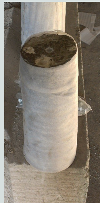
Tapered concrete cylinder with debonding agent
