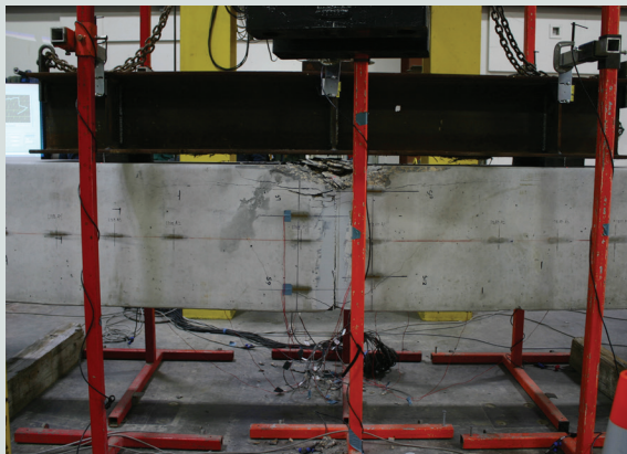
Figure 11. Failure mode in full-scale spliced pile.
