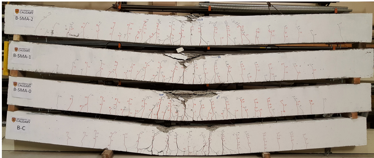
Figure 7. Crack patterns in all beams.
