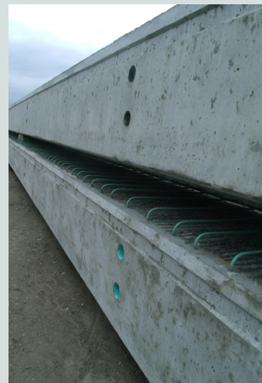
Figure 1. Typical Michigan box beams stored in a precast concrete producer's storage yard.
