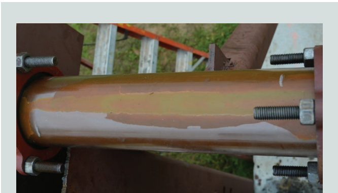
Figure 5: Clear window at top of profile (injection 4).
