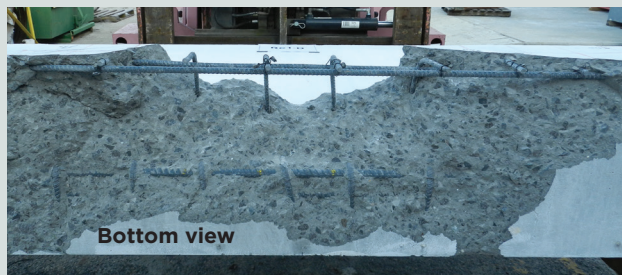
Figure 7. Observed failure surface at midspan, test RS3-M.
