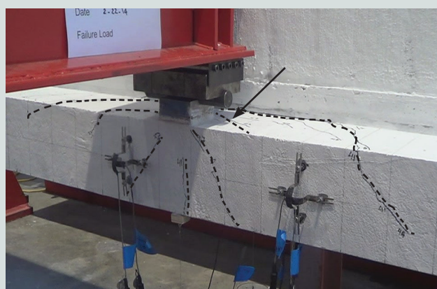
Load = 47 kip, diagonal cracks from back of bearing plate
