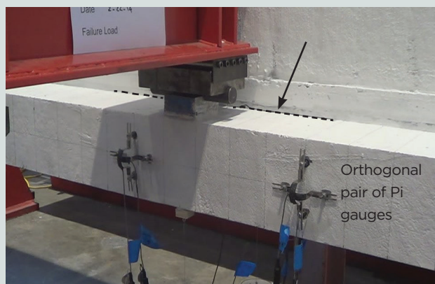
Load = 35 kip, cracks at ledge-to-web junction
