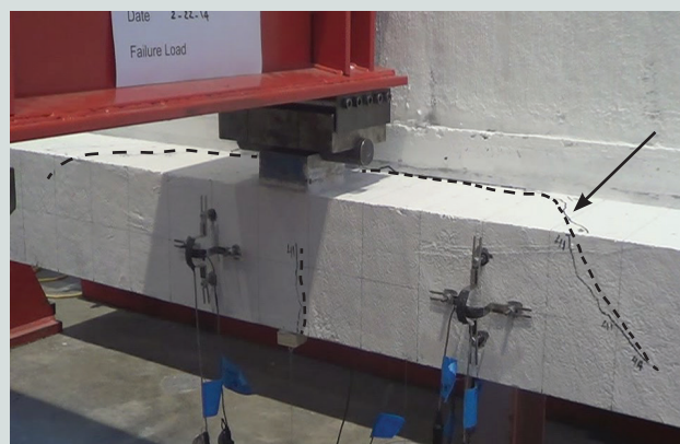
Load = 41 kip, diagonal cracks at top and front ledge face
