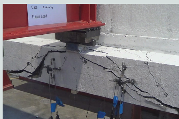
Load = 50.6 kip, failure occurred
