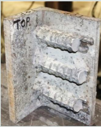
Fractured anchorage bars from lower left connection to center column
