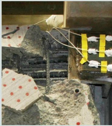
Splitting failure and spalling at upper anchorage bars at right end column
