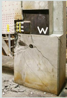
Diagonal cracking of right end column
