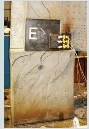
Diagonal cracking of left end column
