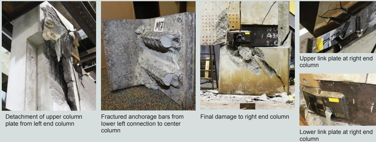
**Figure 8.** Observed failure modes for ordinary moment frame specimen.
