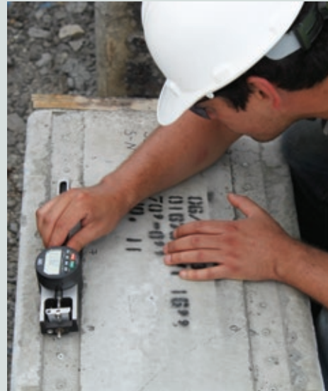
Figure 4. Embedded elements left uniformly spaced points to be measured with a demountable mechanical gauge (left) and measurement of deformations at the surface of the piles (right).
