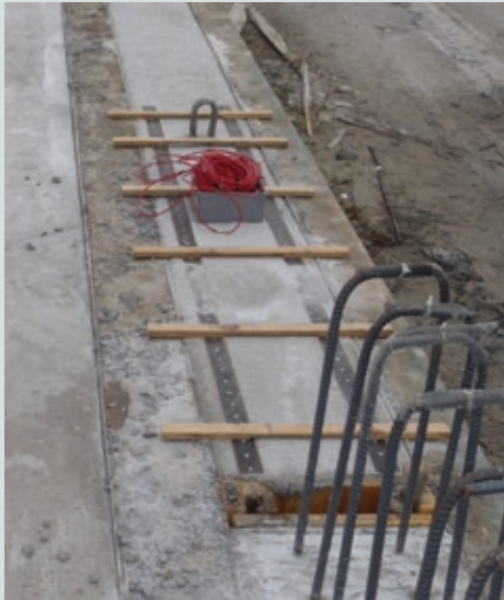
Figure 4. Embedded elements left uniformly spaced points to be measured with a demountable mechanical gauge (left) and measurement of deformations at the surface of the piles (right).
