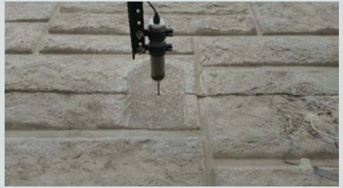
Linear variable differential transformer mounted against face panel
