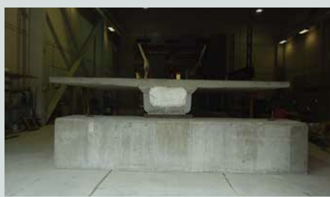
Figure 12. End view of full pretopped box-slab specimen.
