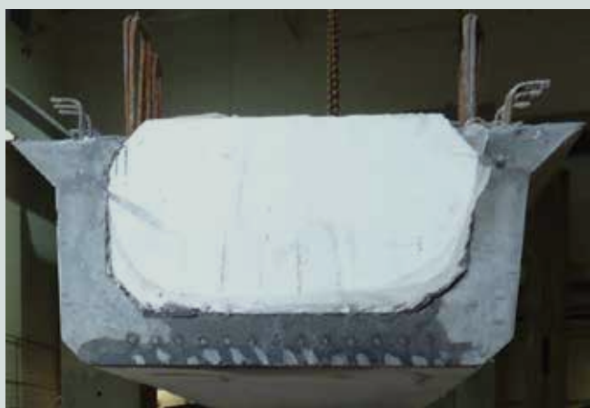
Figure 6. Tub part of the pretopped box beam using two-stage production as delivered to the laboratory.
