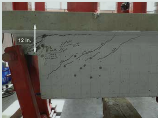
Specimen 8A (12 in. nib height)
