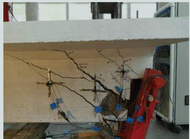
Concrete crushing at the bottom corner
