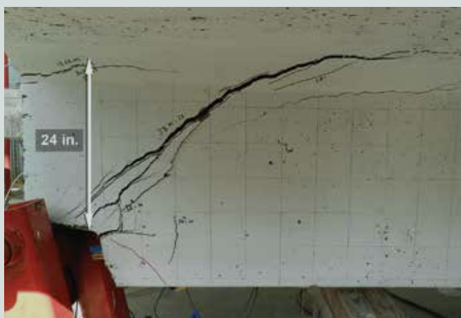
Specimen 8B (24 in. nib height)
