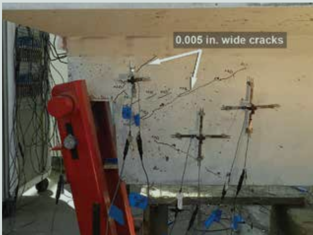
Specimen 1A (vertical L scheme)
